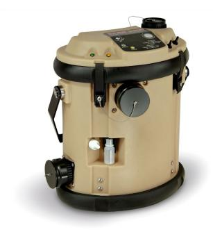
The SASS® 2300 is a highly efficient, portable multistage wetted-wall cyclone sampler that extracts particulates and water-soluble chemical vapors from air and transfers them to a liquid phase for later detection and analysis. This user-friendly sampler has been fieldtested and used in subway systems, public health facilities, nuclear power plants, corporate mail rooms and poultry ranches. It has been proven to possess excellent collection properties.
